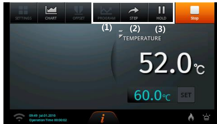
<Fig.3.3.19> Main screen when Program Mode is in operation
