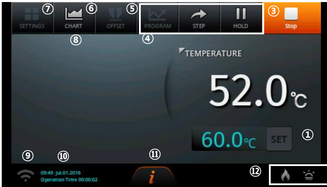
<Fig.3.2.5> Controller for SMART Laboratory Incubator
